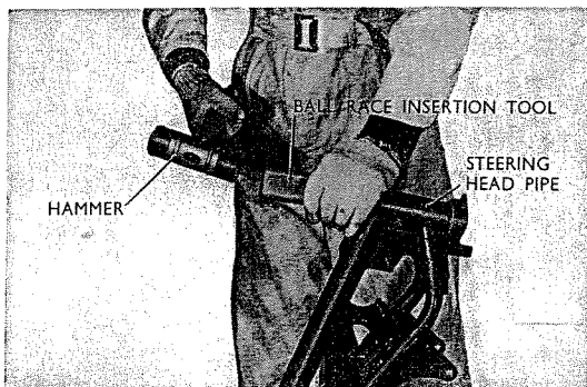
Fig. 4.39 Driving in ball race
